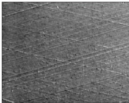
Figure 1. NiC3 Cylinder Bore Cross Hatch
